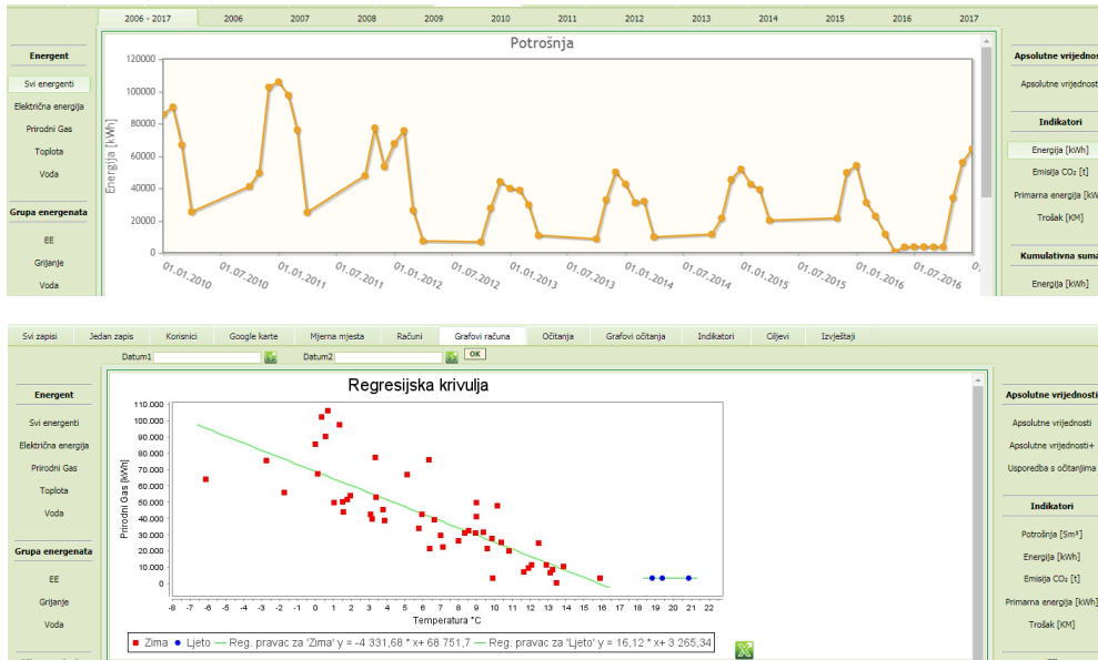
Figure 22 – First figure shows energy consumption of natural gas in kWh in a given time period. The heating periods are nicely recognizable. The second figure shows a linear regression between average monthly outdoor temperatures and monthly natural gas consumption.
